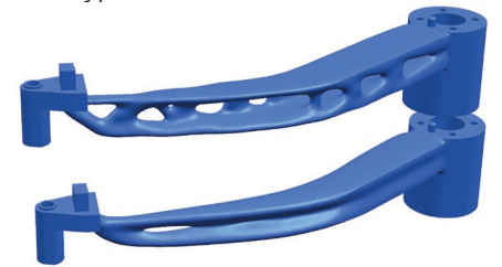
Results from topology optimization may be combined with Convergent Modeling techniques to further refine the design.
